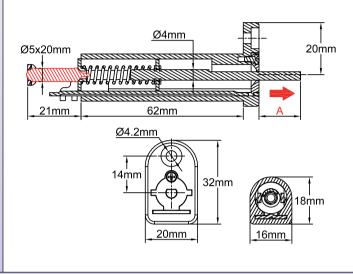
These mechanical thermal actuators are intended to close the fire dampers used on the ventilation ducts. Their large operating force unlocks the spring actuating the damper. Requiring no power supply, these devices are particularly simple and reliable.
